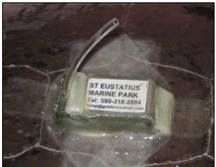
Figure 9. Satellite transmitter fitted to a turtle carapace
