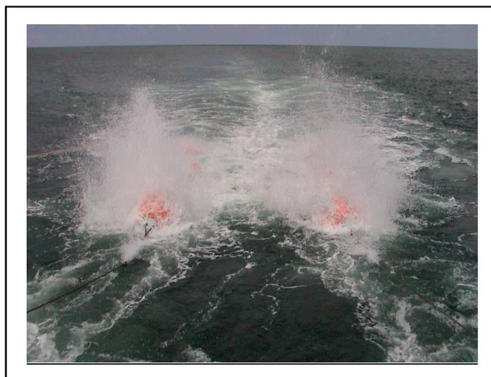
Figure 3.3.6. Source of Fairfield *Speculator* in use during 2002 SWSS D-tag/CEE cruise. The airgun array had a total volume of 1680 in<sup>3</sup>.
