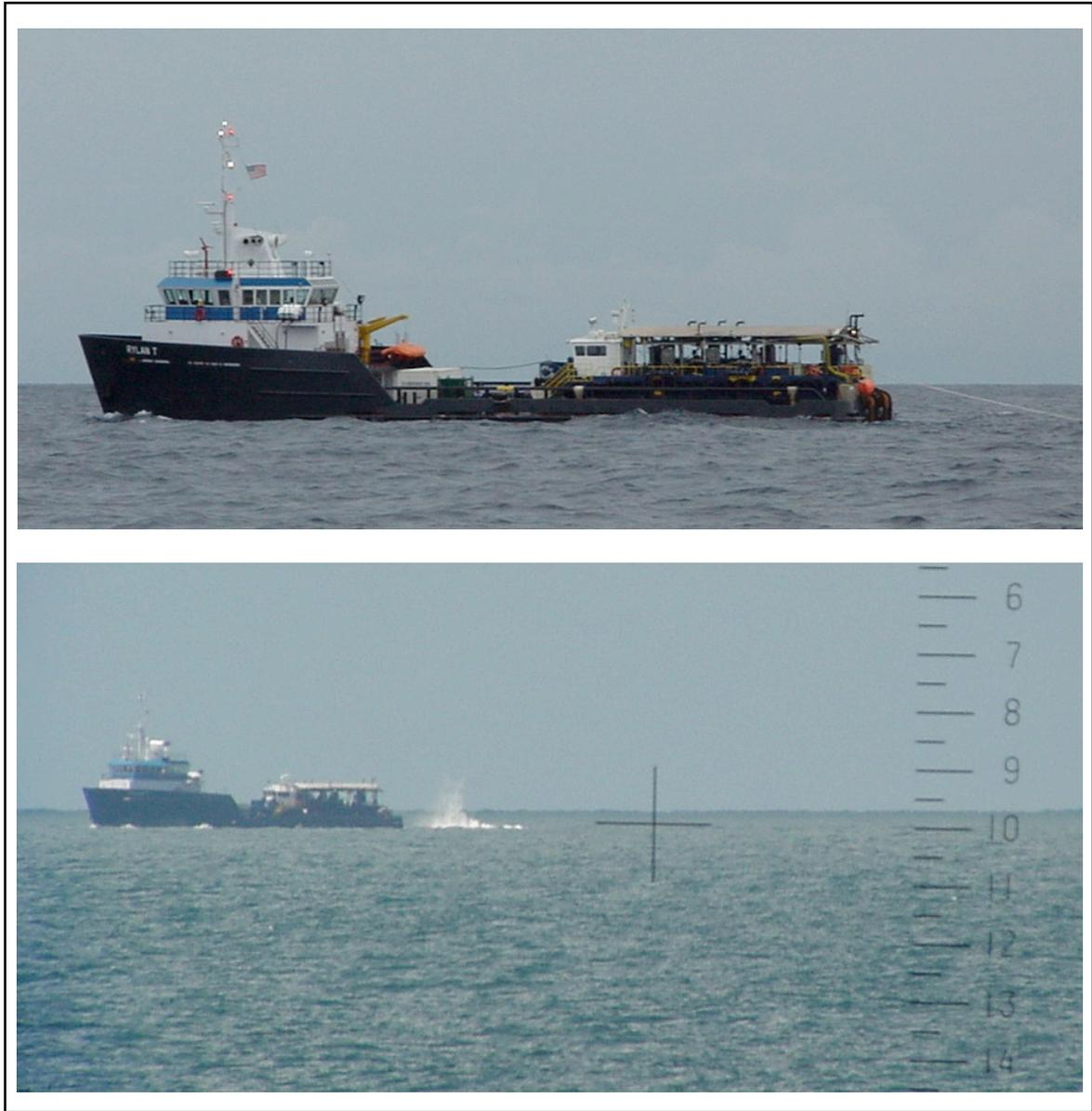
Figure 2.4. Seismic source vessel used on the 2002 D-tag/CEE cruise. The M/V *Rylan T* with the coastal seismic source vessel *Speculator* mounted on the back deck (upper) and airgun action through BigEye binoculars during a 2002 controlled exposure experiment (lower). The cable on the right is the tow cable for the SEAMAP passive acoustic array.
