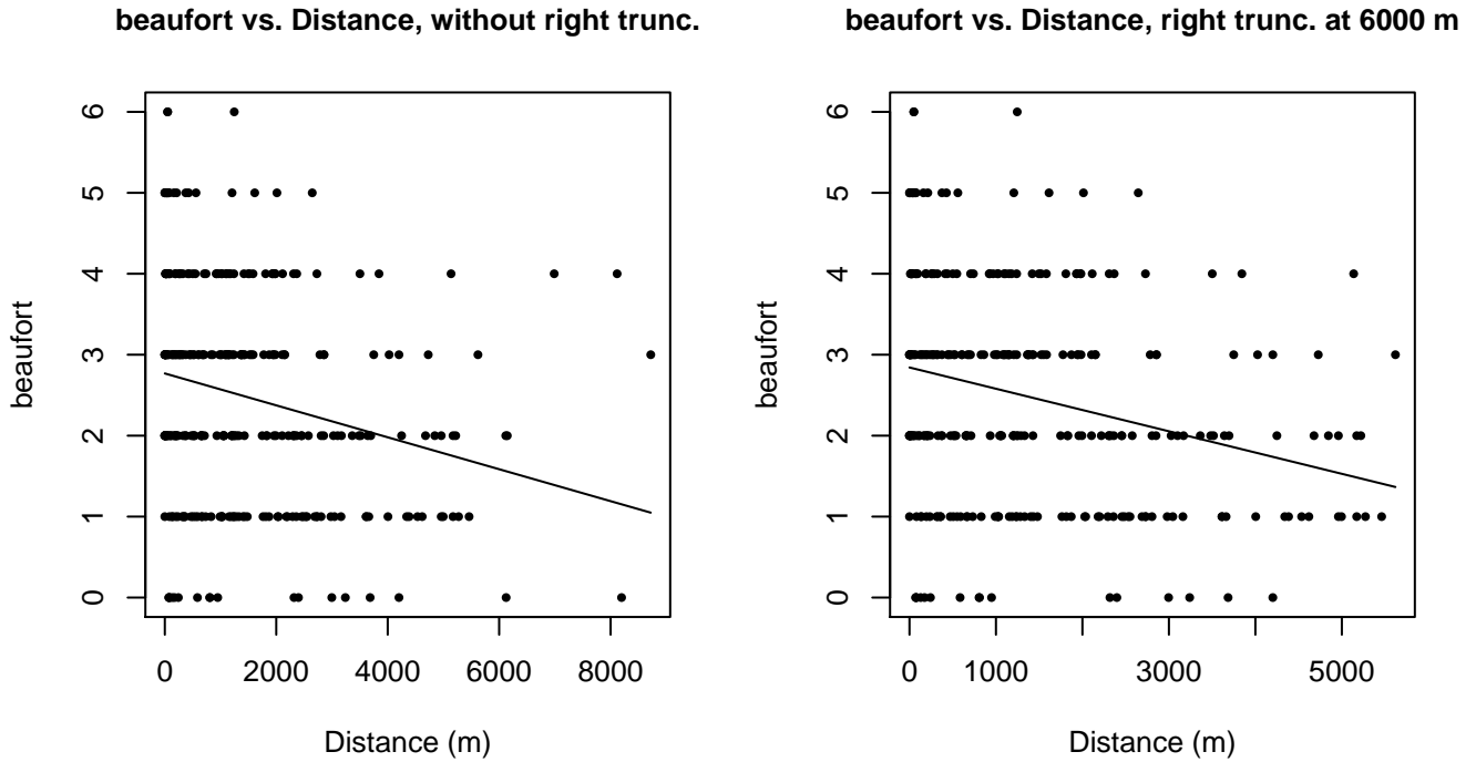
Figure 13: Scatterplots showing the relationship between Beaufort sea state and perpendicular sighting distance, for all sightings (left) and only those not right truncated (right). The line is a simple linear regression.
